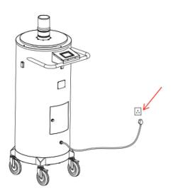
3. Select on the touch screen: power on delay time and sterilization time, then press the start button, please leave the room immediately after hearing the alarm sound of the warning light, pay attention (in the use of ultraviolet lamp irradiation disinfection, should not be present, in order to avoid the direct exposure of ultraviolet ray to the eyes and skin injuries).
