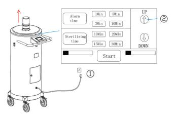
4. Press the "down" button on the touch screen to hide the tube in the light box. Turn off the power and plug off the UVC light, as shown in the figure below:
