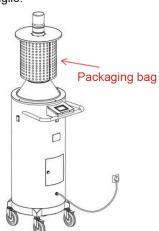
2. Plug in the UVC light. Then press the "up" button on the touch screen to make the tube rise to the top, as shown in the picture below:
