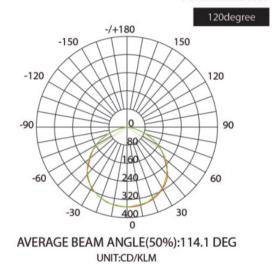
All published Luminaries photometric testing performed to IESNA LM-79-08 standards by a NVLAP
