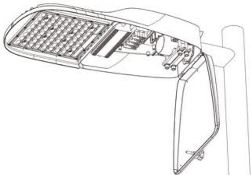
8. Cover the fixture cover and tighten the thumb screw to complete the installation.
