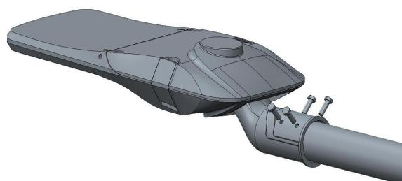
**Step3: Loosen the screw, adjust the angle required for the maximum angle is 15 °**
