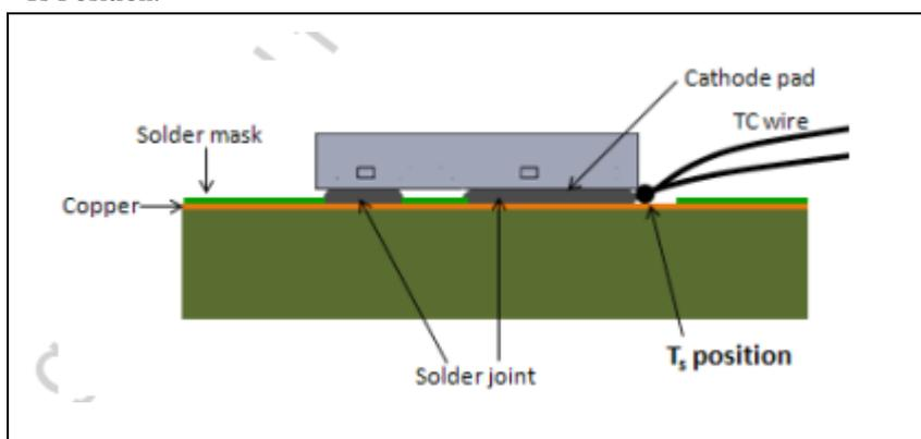
Thermocouple Location on Temperature Measurement Point (TMP):
